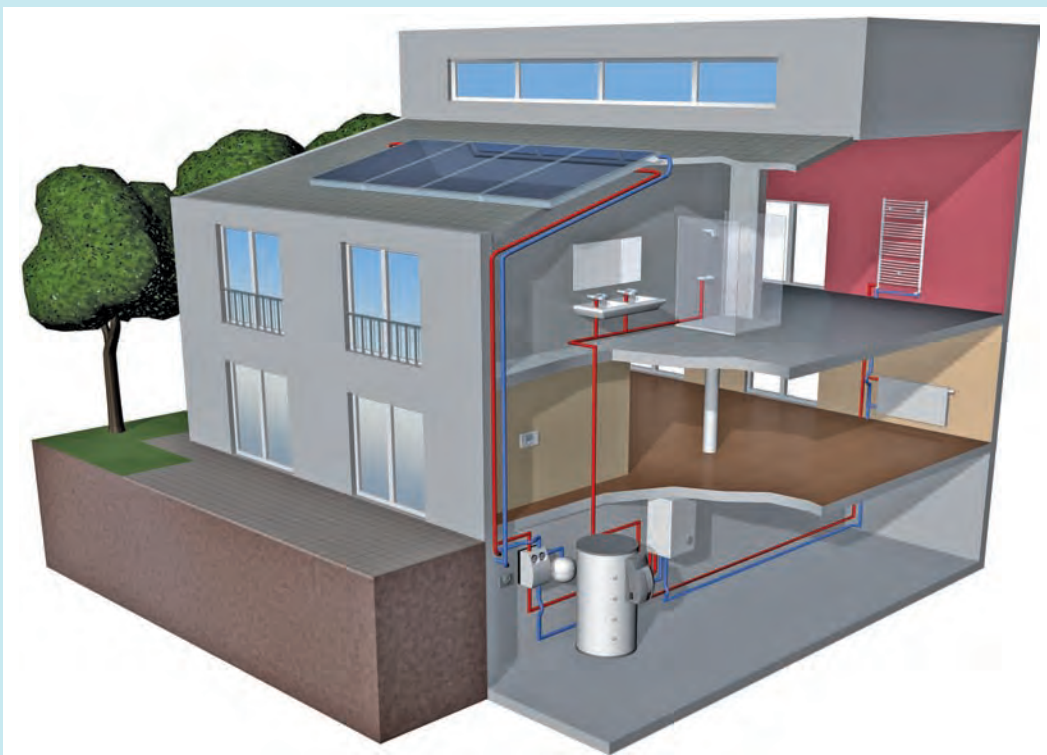
A total heating system with a Baxi wall-mounted boiler in the basement
